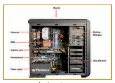
Fig. 6. Structure of a computer
