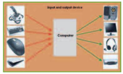
Fig. 7. Input and output devices of a computer
