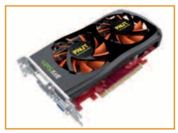
Fig. 11. GeForce GTX 560 TI graphics card
